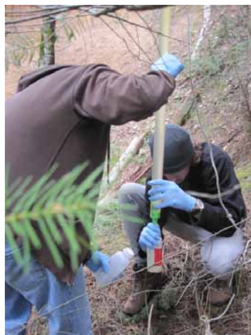
Figure 19. Collecting Water Sample from an Access Shaft Using a Bailer
