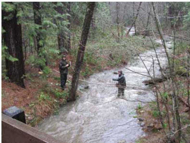
Figure 16. Discharge Measurement at Road 1, Humbug Creek Discharge was measured using the Marsh McBirney flow meter model 2000 with top-setting wading rod. (K. Landrum (left) and H. Nepal (right) in photo; photo taken on March 15, 2011 by C. Monohan.)
