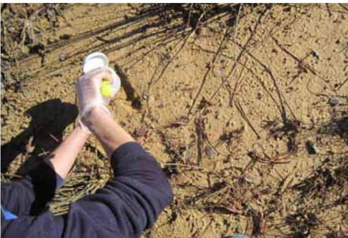
Figure 18. Confirmation Soil Samples from the Malakoff Diggins Pit
